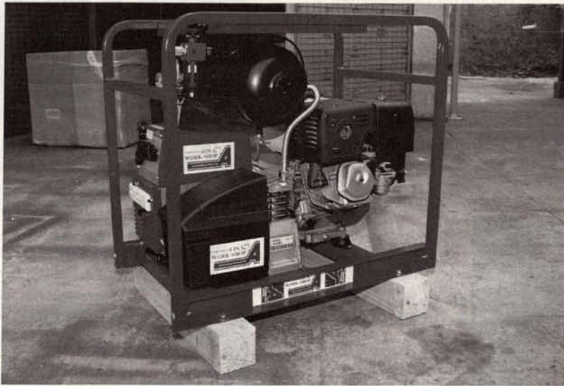
The latest Advanced Power Products range of welder-generators and four in one workstations offering generator, battery charger, welder and air compressor and provide the resources to undertake repairs or maintenance tasks on the farm, workshop, mine or construction sites. A choice of eleven different models and petrol or diesel engine powered versions are available. The model shown offers 7kVa power, 100 amps welding, 10cfm compressed air plus battery charging.
